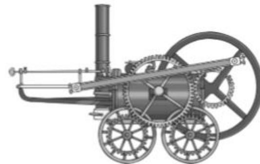
Richard Trevithick's unnamed locomotive carried 10 tons of iron over a distance of 16km at the Pen-y-Darren Ironworks in Wales.
